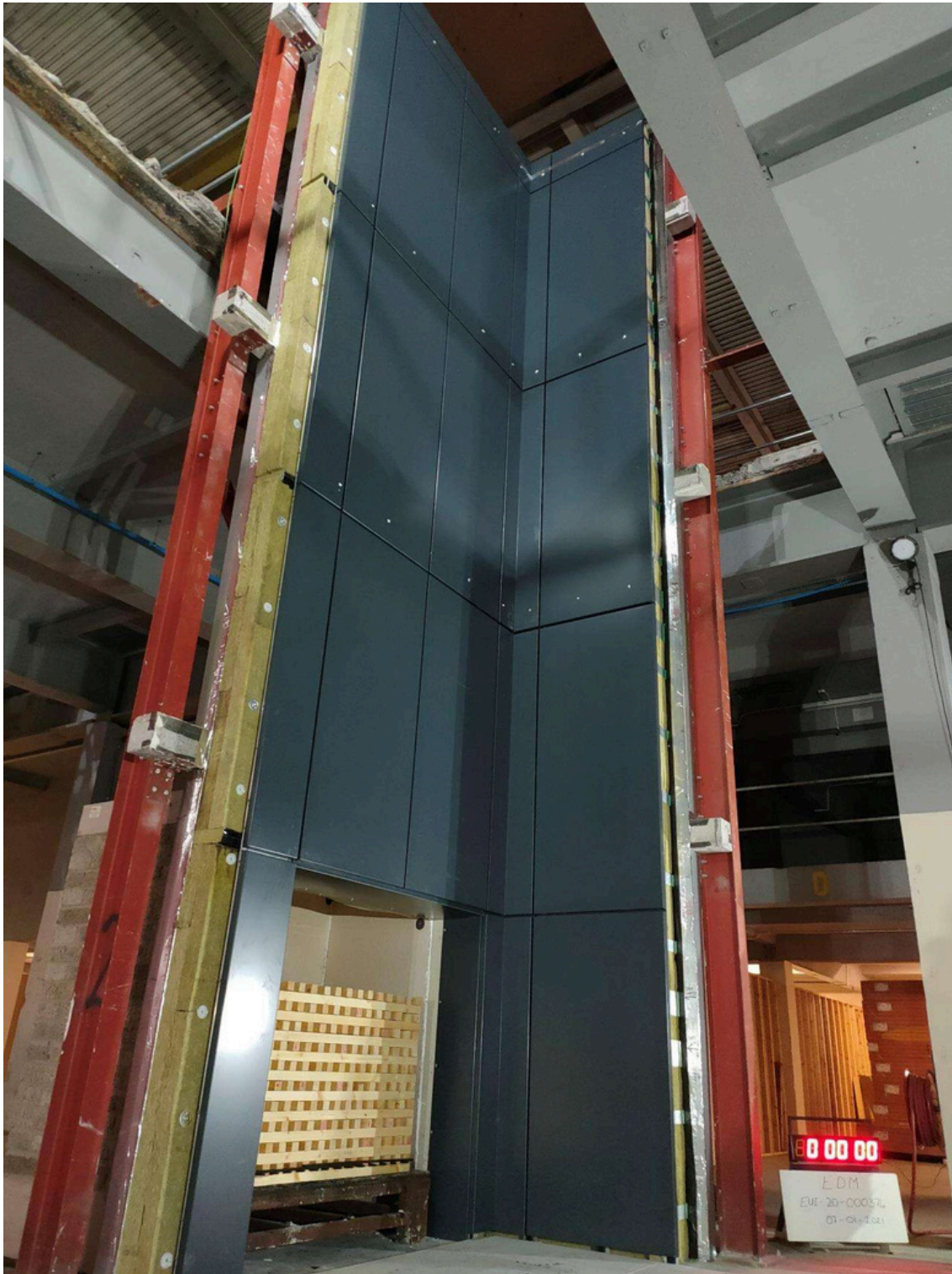
Figure 26. Cladding system before the test.
